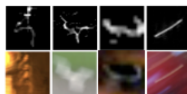
Figure 10: Top row: Inferred blur kernels from four real images (the cafe, fountain and family scenes plus another image not shown). Bottom row: Patches extracted from these scenes where the true kernel has been revealed. In the cafe image, two lights give a dual image of the kernel. In the fountain scene, a white square is transformed by the blur kernel. The final two images have specularities transformed by the camera motion, revealing the true kernel.
